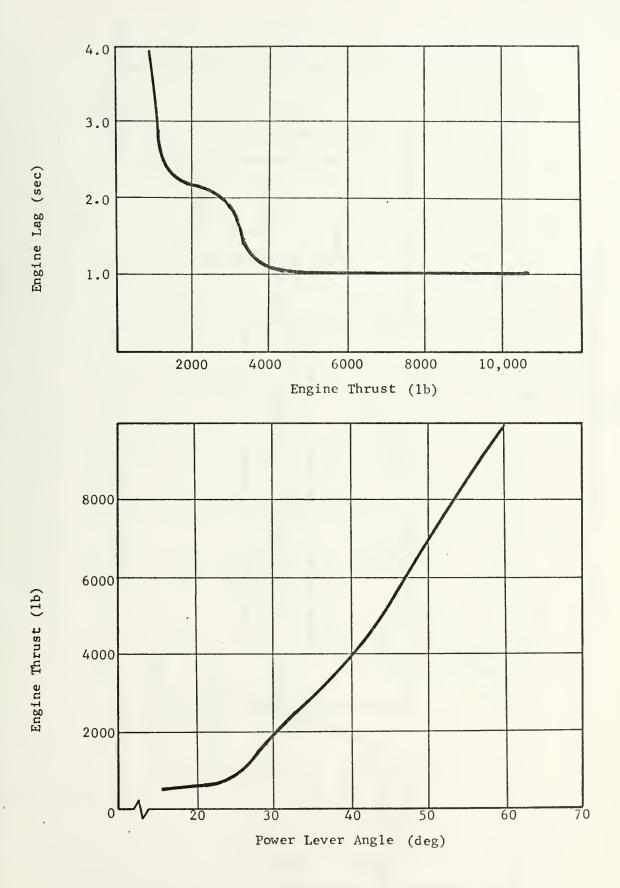
FIGURE 2. TF41-A-2 ENGINE CHARACTERISTICS
