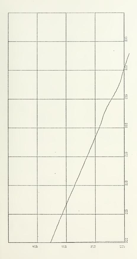
APPROACH PROFIL TIME JUDD X-SCALE=5.00F+00 UNITS INCH. Y-SCALE=2.00E+02 UNITS INCH. A-7E AIRCAAFT CARRIER ALTITUDE RESPONSE US
