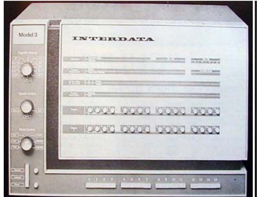
The 1968 Interdata Model 3 Control Computer could handle 16 and 32 bit instruction word lengths, had 1024 bytes of memory expandable to 65,536 bytes, 2 microseconds cycle time, and had 16-bit arithmetic and 16 general registers. It sold for about \$6,000.
