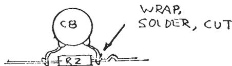
3. Install and solder R2-C8, R14, and D1 as shown below. Install the formed leads into the board with the unformed leads vertical. Position R2-C8 so that the body of C8 is parallel to the board edge and oriented away from C1.
