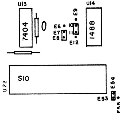
Jumpers for the Main logic board for use with another computer (Direct Wire) & the ALTEST DB25 connector
