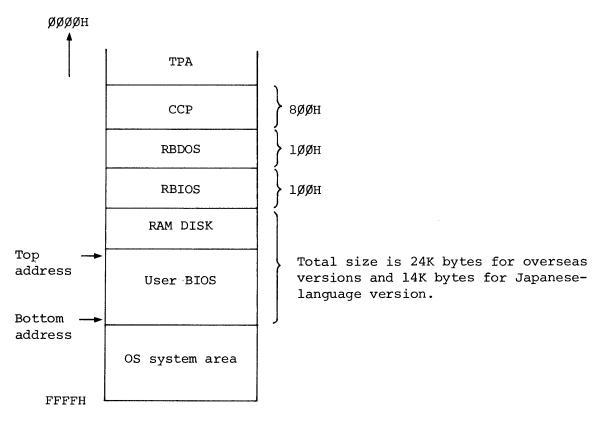
Either the BIOS or interrupt processing routines can be extended by loading their extended portions in the user BIOS area.
