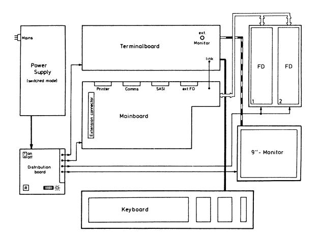
Figure 1. P2000C - System Architecture
