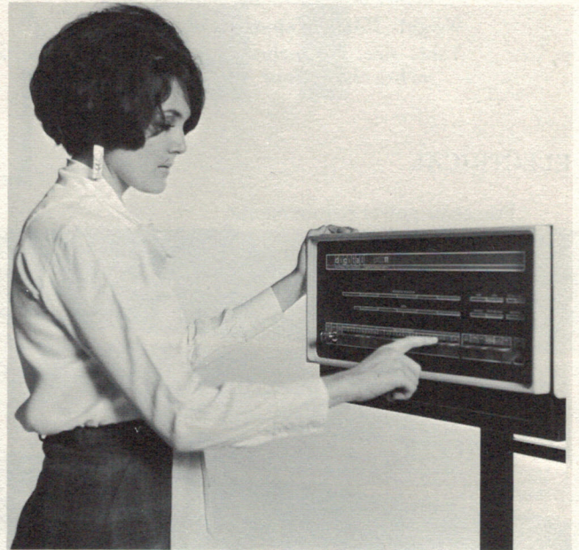
The plug-in console board with modular construction is supplied in the basic 11/20 configuration. In addition to aiding programming, console contributes to ease of maintenance on the PDP-11.
