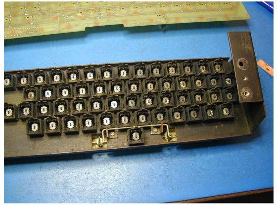
And here is the pcb showing the reed switches mounted vertically and the diode matrix for encoding each switch:
