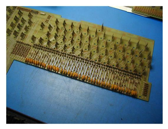
The reed switches can now be inspected and replaced if necessary. The top wire is welded to the metal bracket, but can be separated with a pair of sharp diagonal cutters. The new switch can be soldered instead.
