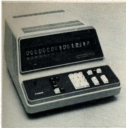
Canon 161 is a self-contained unit with Nixie-tube display and integrated circuits.
