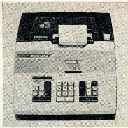
Operators (+, -, etc.) are printed in red on paper tape of Monroe's Epic 3000.
