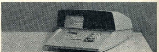
This microelectronics calculator by Victor employs 30 MOS (metal-oxide-semiconductor) devices for circuit reliability.
