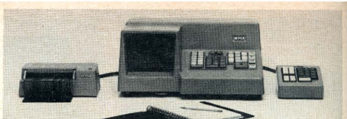
Wyle Scientific calculator uses a cathode-ray-tube display.
