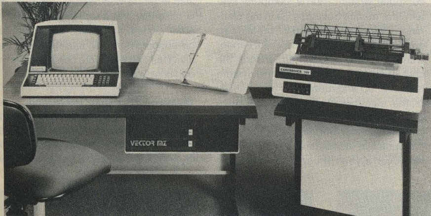
Vector Business System—MZ Computer with dual floppy drive, MT Terminal, and Centronics 702 Printer.
