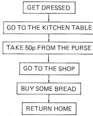
Each box contains an instruction, and the arrows show the order in which the instructions are executed. Well, that looks pretty simple and neat. Now that the flow diagram is drawn on paper we can check it by going through the boxes one by one and asking ourselves: Can the child (or the computer) do this?
