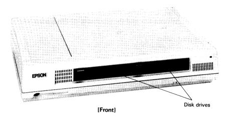
The main unit includes the system's  $\mu$ PD780-1 CPU (Z80A compatible), the main memory RAM chips, twin disk drives, interfaces for peripheral equipment, and the computer system's power supply, and is connected to the display monitor and keyboard through DIN connectors. All QX-10 power is controlled by a single switch on the back right side of the main unit.
