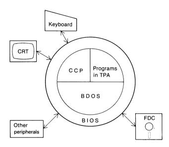
CCP reads and interprets commands input from the keyboard. BIOS provides an interface between peripheral devices and the other modules of CP/M. BDOS performs disk file management, and is the nucleus of CP/M. BIOS and BDOS are explained in more detail in Chapter 7. For further details, refer to any of the various books available on CP/M.
