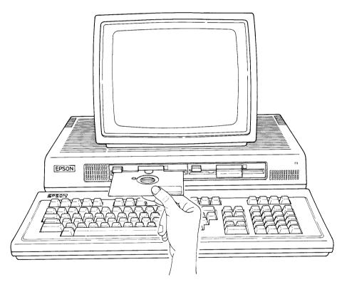
Push the disk in until it reaches the back-stop, then continue pushing until it clicks into place. (If the disk does not go in smoothly, do not apply force; pull it back out and start over, being careful to properly align it with the drive entrance. Forcing the disk can damage it, resulting in destruction of its contents, improper drive rotation, and a variety of other problems.)
