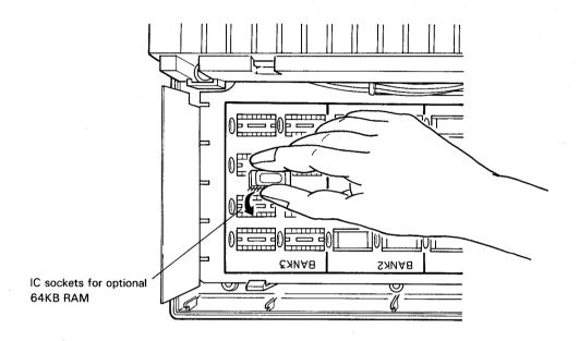
These RAM chips are supplied as standard equipment on units with the German keyboard.
