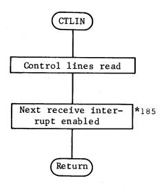
\*185 Enable Interrupt on Next Rx Character command sent to the  $\mu\text{PD7201}$ .
