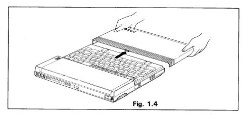
Place the thumb of each hand on the top of the cover, with the other fingers on each side of the cover. Press gently with the index fingers to release the catch in the top centre (see the arrow in the diagram). Now pull the whole cover towards you using the both hands so that it slides off.
