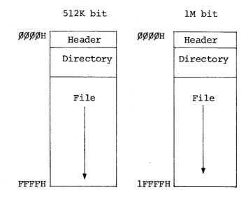
The capacity field at the second byte of the header contains different values for different ROM types.
