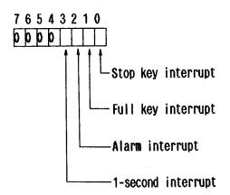
(Interrupts are enabled when the corresponding bits are set to 1, and disabled when reset to 0.)
