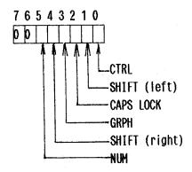
(Each bit is set to 1 if the corresponding key is pressed down at power off time.)
