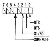
(DTR and RTS are active when the corresponding bits are set to 1, and  $\overline{\rm SI/SO}$  and  $\overline{\rm XON/XOFF}$  controls are specified when set to 0.)
