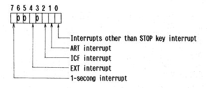
(A 1 in a bit position disables the corresponding interrupt and a  $\emptyset$  has no effect.)
