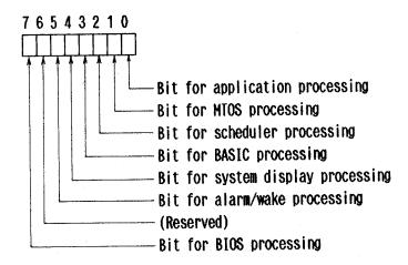
(When each bit is set to 1, the corresponding type of processing is disabled.)
