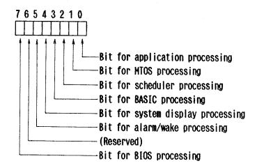
(When each bit is set to 1, the corresponding processing is disabled.)
