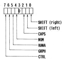
(Bits 5-2 are set to 1 when the corresponding modes are set to ON; other bits are set to 1 when the corresponding shift keys are pressed.)
