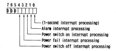
(When a bit is set to 1, the corresponding type of processing is executed.)
