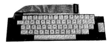
53 key non encoded keyboard (keys are decoded by polling from the operating system, each key has a place on the cross matrix) designed to plug into CUBIT, CUNINE or CUMOT single board computers. The new CUBOS operating system for the 6502-based CUBIT supports this keyboard, which, together with CU-MEM, Acorn 40 column video card and Acorn Atom BASIC make up the Industrial Control Unit described on page 1.5.
