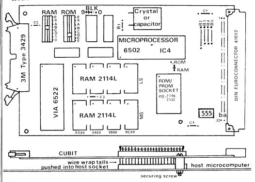
CUBIT is a Eurocard sized (100mm  $\times$  160mm) microprocessor  $\,$  module with four main functions.
