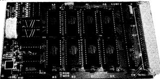
CU-MEM is a Euro-card using the standard Acorn bus, with eight 28 pin sockets, each of which can take the industry standard range of 24 and 28 pin memory devices, offering RAM, ROM and PROM options. The sockets are arranged in two banks, which can be individually selected for their position in memory (in 8K divisions) and for the type of memory device used. This allows the popular option of a bank of RAM (up to 8K) and a bank of PROM (up to 16K using the 2564 or similar).
